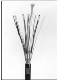
31 core camera cable with kevlar strength member, XLPE cores, and polyurethane elastomer jacket.
