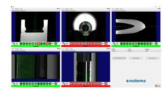
The user interface provides easy access to inspection results, settings and statistics. Real time statistics can be stored into a customer specific text file for data export. An update to the AAI 3.0 user interface is the possibility to simply configure new product characteristics.
