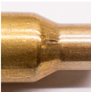
Wrinkle at chest detected with line scan camera.
