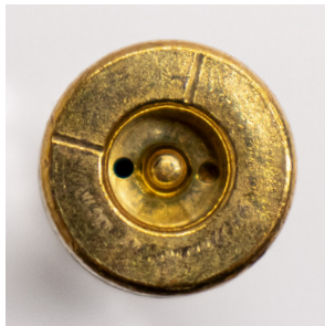
Missing firing hole easily detected through back light.
